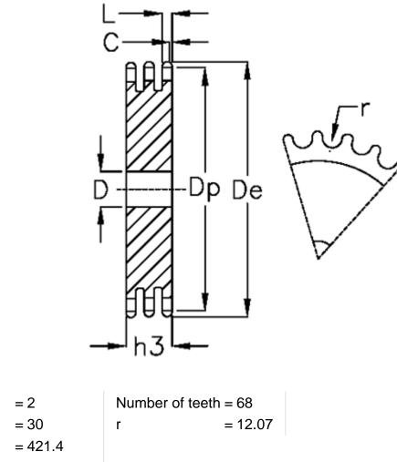
C = 2 D = 30 De = 421.4 Dp = 412.49 For chain size =  $3/4 \times 7/16$ For chain type = 12 B-3 h3 = 49.8 L = 10.8
